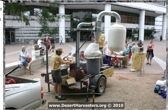
Desert Harvesters' Meadows #5 gas-powered, portable hammer mill at a public milling event in downtown Tucson. Community members bring their own mesquite pods and volunteers operate the mill. Pods are passed through a #4 screen and flour is collected in the first barrel and fines are collected above the cyclone.
